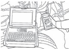
**Figure 5. Measuring the Coolant and Air Temperatures**
