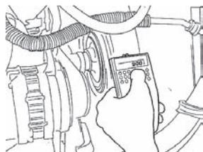
**Figure 4. Measuring Fan Blade Speed with Digital Photo-Tachometer**
