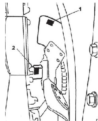
**Figure 1 Placement of Reflective Tape**
