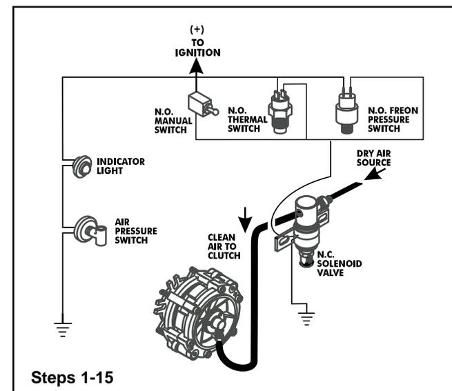
6. Connect the Red (12 Volt) or Green (24 Volt) lead of the N.C. Solenoid Valve to one terminal of the N.O. Thermal Switch.
